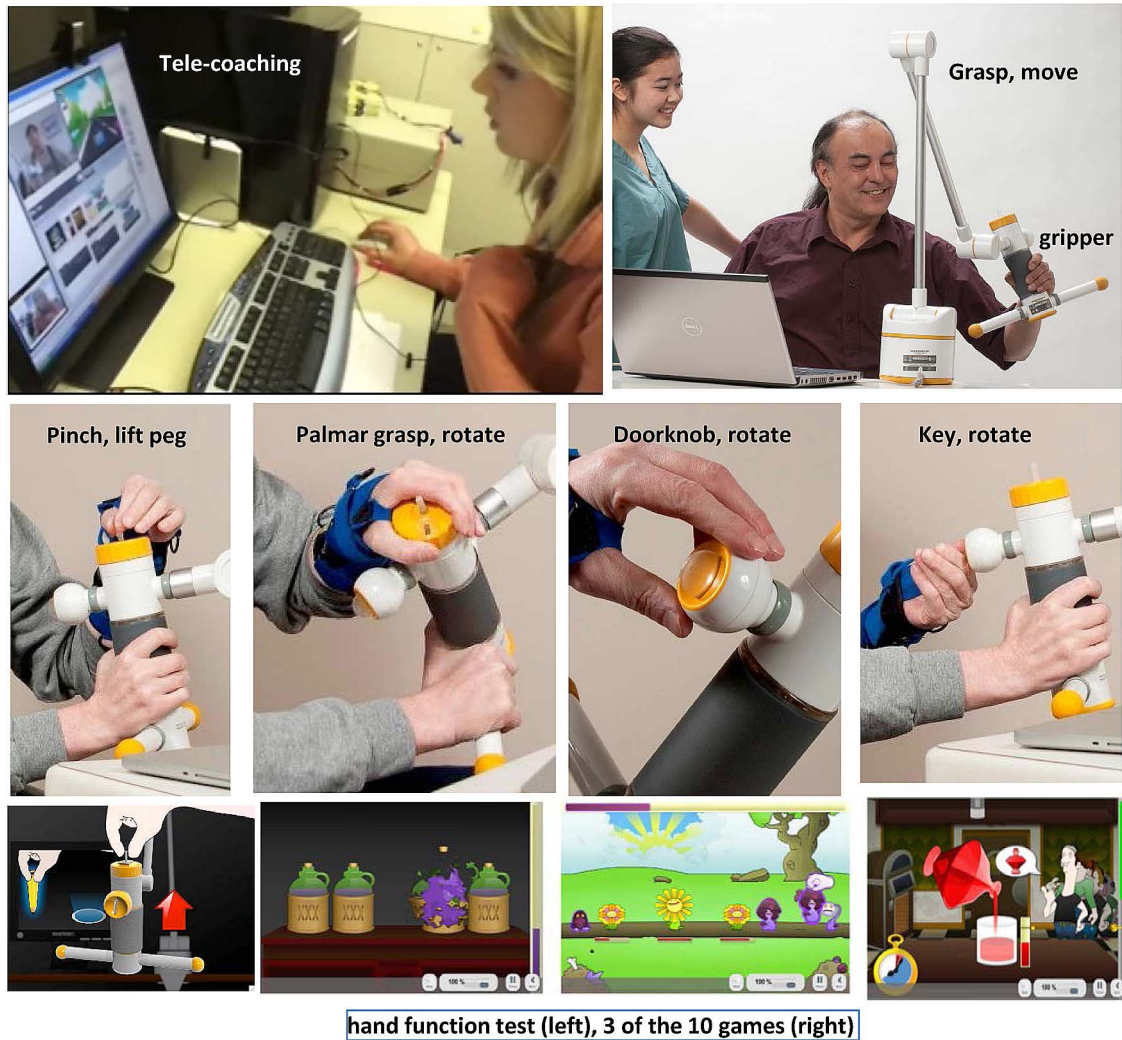
Fig. 2. FES-assisted exercise therapy on the ReJoyce workstation. Top: Tele-coaching and exercise training; Middle: Dexterous tasks performed on the device. Bottom: Screen-shots of hand function test (far left) and examples of computer games available.
